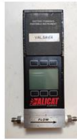
ELECTRONIC FLOWMETER (RANGE: 1 - 750 ML/MIN) (TESTED) CS_OT_00005-3000
