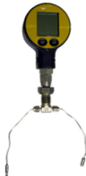
ELECTRONIC MANOMETER ASSY (RANGE: -1 À 2 BARS (RELATIVE PRESSURE)) (TESTED) CS_SE_00007-MANO
